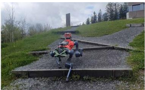
Fig. 2. A hike on the Etzel mountain in Switzerland, completed by ANYmal with our locomotion controller. The 2.2-km route—with 120 m of elevation gain and inclinations up to 38%—encompasses a variety of challenging terrains [(A) to (I)]. ANYmal reached the summit faster than the human time indicated in the official signage and finished the entire route in virtually the same time as given by a hiking guide (47).
