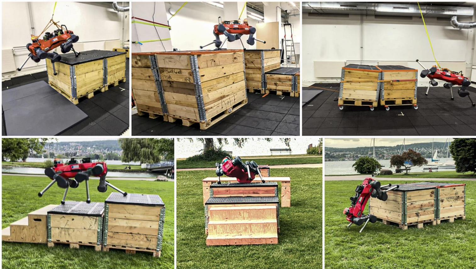
Fig. 1: Deployment of the pipeline on the quadrupedal robot ANYmal D. The robot performs highly dynamic maneuvers and makes contacts with its limbs where necessary.
