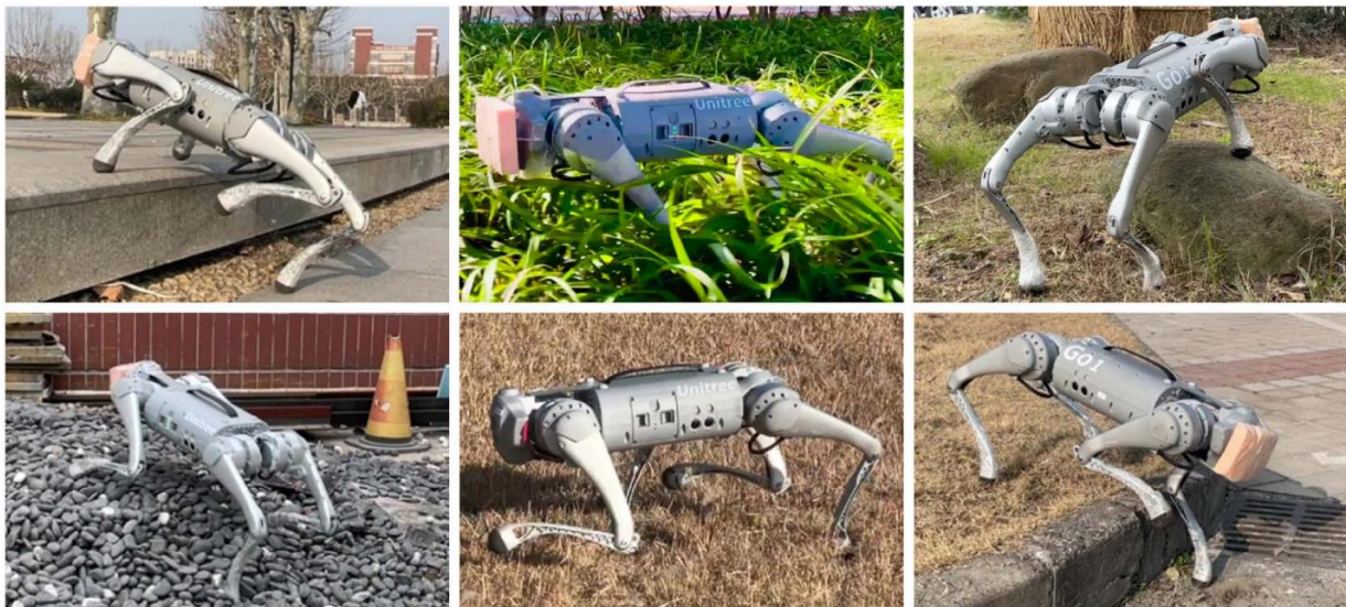
Fig. 1. Our robot can achieve robust locomotion over challenging terrains and agile locomotion over natural terrains. The robot can successfully traverse curbs, stairs, rocky and vegetation while running and spinning at high speed over natural terrains. Whether on even or complex terrains, at high or low speeds, the emergent behaviors learned by our robot exhibit a natural gait and smooth motion.
