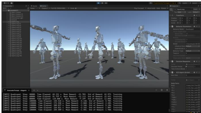
Figure 2. The training interface. The robot is trained parallelly with CPU.
