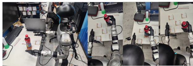
Fig. 6. End-to-end grasping demonstrations of the Unitree G1 at five positions within the workspace.
