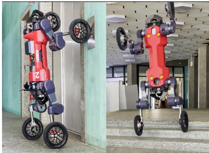
Fig. 1. Quadruped-humanoid transformer ( https://youtu.be/kEdr0ARq48A ) with a time-lapse from left to right of a stand-up and sit-down motion (top image), obstacle negotiation (middle image), and indoor navigation (bottom images). The former skill and the humanoid navigation on two legs are achieved through traditional RL training with a task reward formulation. Instead of tuning the sit-down skill, we can reverse the playback of the stand-up motion and use it as a motion prior that helps the robot discover feasible sit-down behaviors avoiding tedious reward function tuning.
