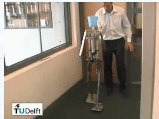
Fig. 2. Three level-ground powered walking robots based on the ramp-walking designs of Fig. 1. (A) The Cornell biped. (B) The Delft biped. (C) The MIT learning biped. These powered robots have motions close to those of their ramp-walking counterparts as seen in the supporting on-line movies (movies S1 to S3). Information on their construction is in the supporting online text (9).
